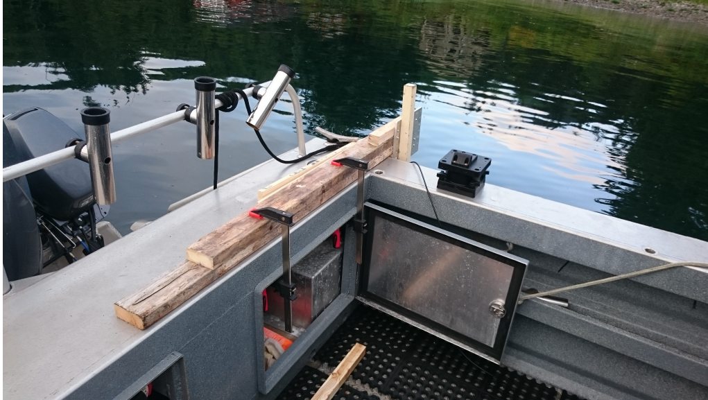
Figure 1: Horizontal portion of measurement arm clamped to boat stern. This portion of the arm is fabricated on-site, with available materials to reduce the amount of equipment during travel.
