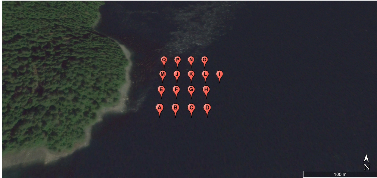
Figure 4: Google Earth view of measurement points. A measurement grid is set up in the area known to have high flow velocities.
